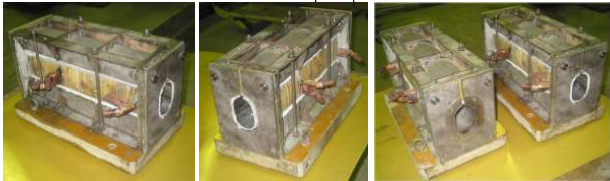
Fig. 1 Inductors for aluminum extrusion
