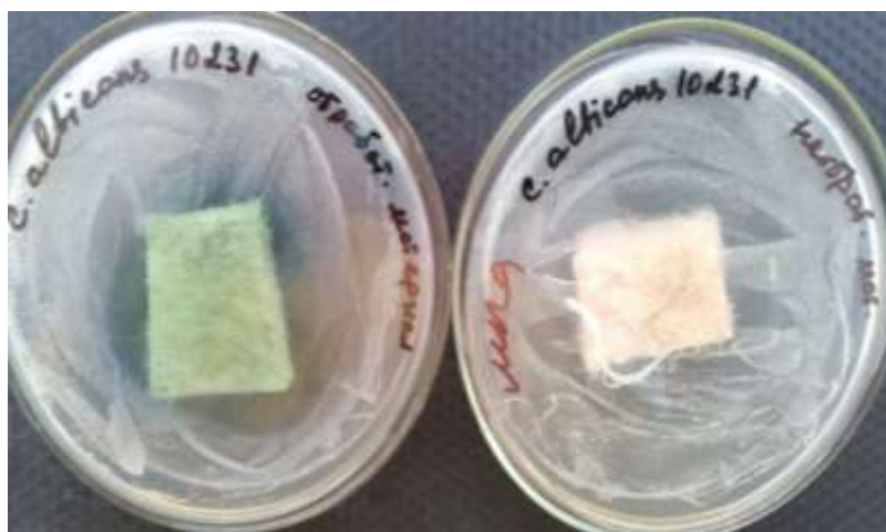
Figure 3 - Growth retardation zone of the test strain C. albicans ATCC 10231 (experimental and control sample)
