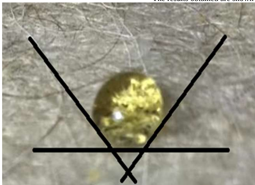
Figure 2-Images of a drop of water on the surface of a non-woven material treated with an organosilicon compound and MK
