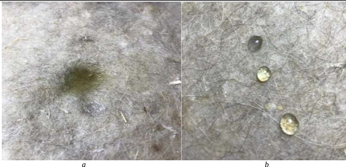
Figure 1-Images of a drop of water on the surface of a non-woven material: a-the starting material; b-the material treated with an organosilicon compound and MK
