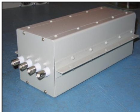
Fig. 2. The electronic equipment for signals receiving from the vector receiver and transferring it to a personal computer
