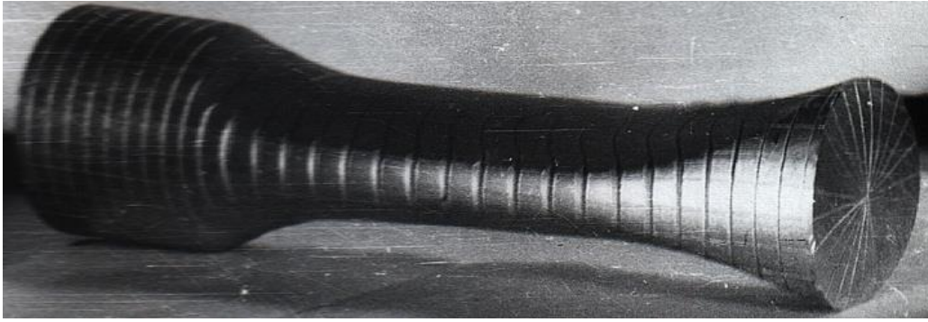
Fig.1 –A sample after rolling with increasing and decreasing compression
