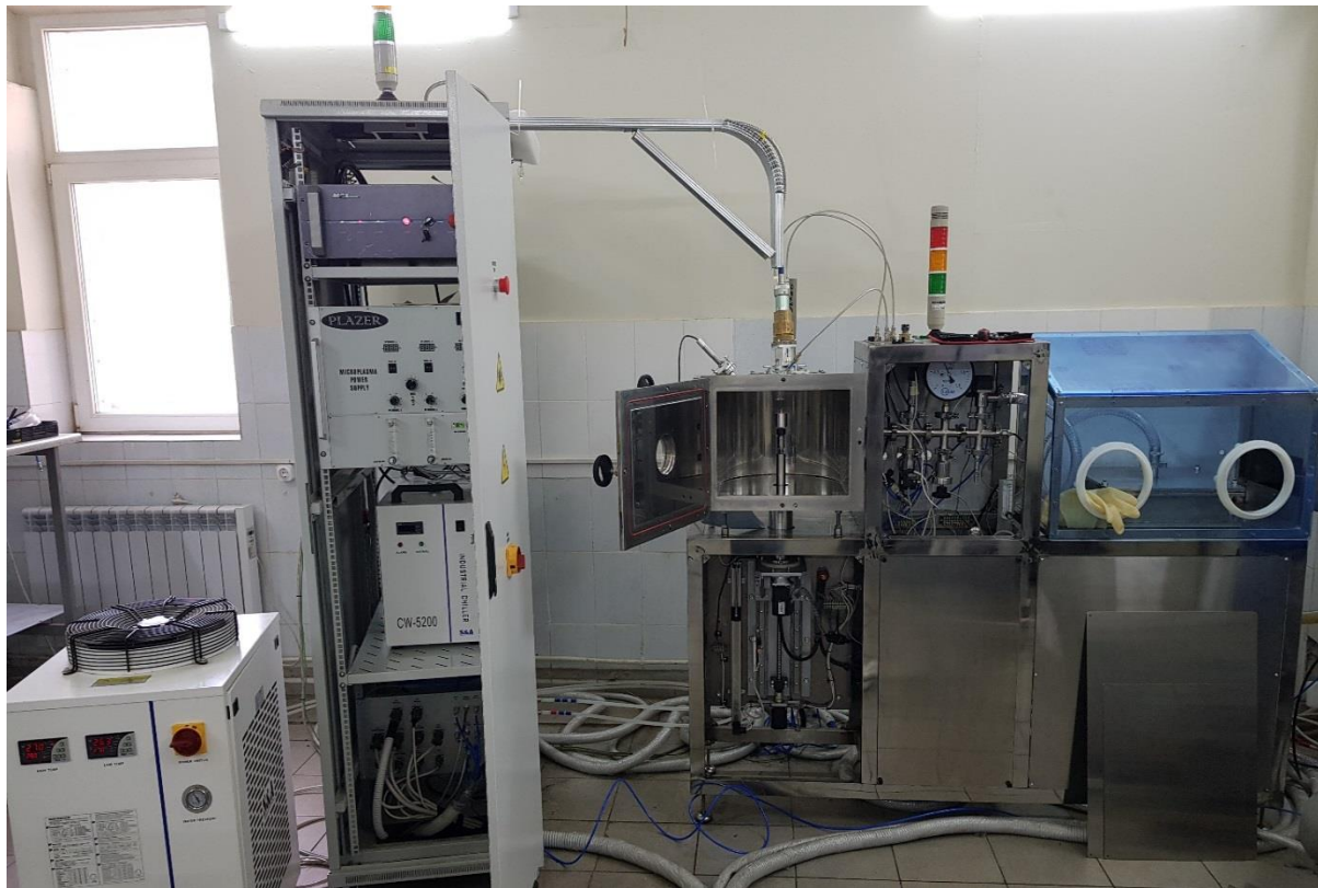
Fig. 1. The appearance of the research and industrial complex for welding thin-walled products of the space industry from light high-strength alloys.
