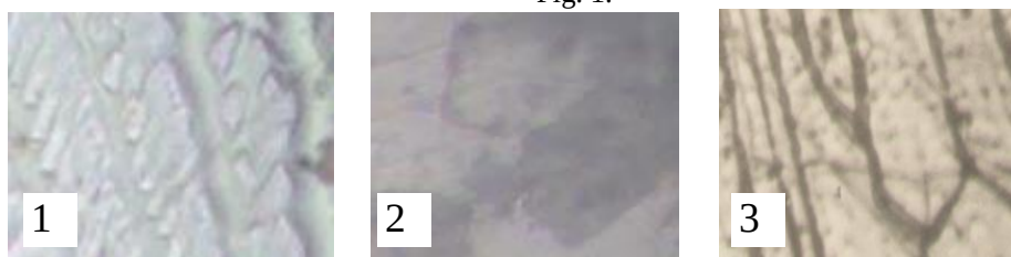
Fig. 1. Microstructures of alloys of the \text{As}_2\text{Se}_3 - \text{TlGaS}_2 system. 1-20 mol %, 2-60 mol %, 3-92.5 mol % \text{TlGaS}_2 .
