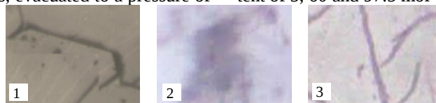
Figure 1. Microstructures of \text{TlAsSe}_2 -InSe system alloys. 1-5 mol %, 2-60 mol %, 5-97.5 mol % InSe.
