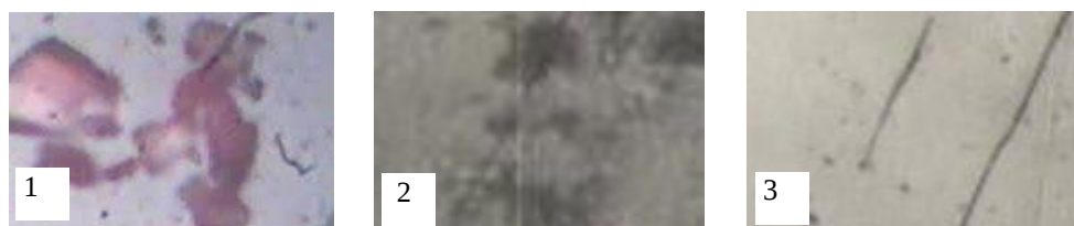
Fig. 1. Microstructure of alloys of the \text{SrIn}_3\text{-SrSe} system. 1-30 mol %, 2-70 mol %, 3-97 mol % SrSe.
