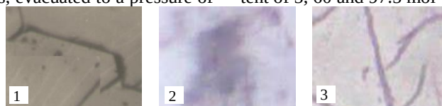
Figure 1. Microstructures of \text{TlAsSe}_2 -InSe system alloys. 1-5 mol %, 2-60 mol %, 5-97.5 mol % InSe.
