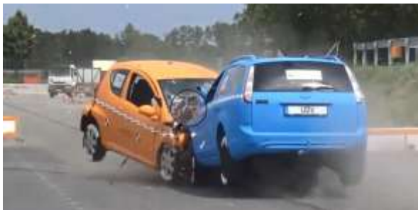
Figure 5 - Maximum penetration and impact impulse (rear view)
