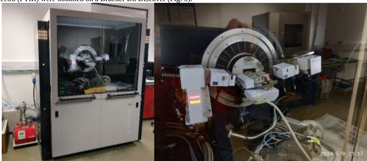
a) Figure 5. - Diffractometer (a); its working chamber (b)
