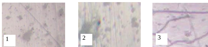
Fig. 1. Microstructure of \text{AsS-Cu}_2\text{Cr}_4\text{Te}_7 alloys. 1–40 mol. %, 2–70 mol. %, 4–90 mol. % \text{Cu}_2\text{Cr}_4\text{Te}_7 .
