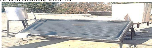
Figure 2. Experimental setup of the forced-convection solar dryer utilized for persimmon dehydration, comprising a flat-plate solar collector, a drying cabinet, and an exhaust fan [34].
